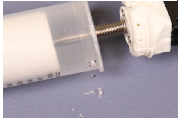
Remove excess Plastic
