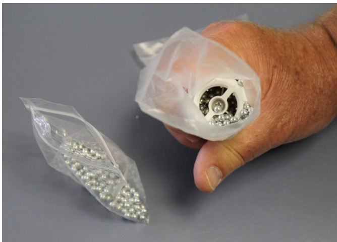
Fill the Cylinder with BBs
