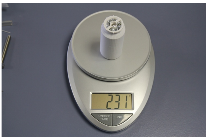
Cylinder with BBs should weigh 220-232g
